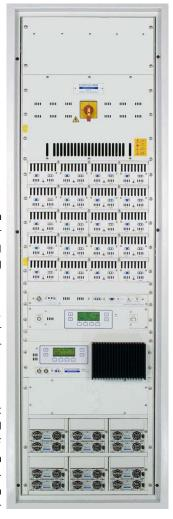
Outputs from the 19 power modules are combined via the 19 way N way combiner. The combined RF output is then fed to the output coupler and harmonic filter.
